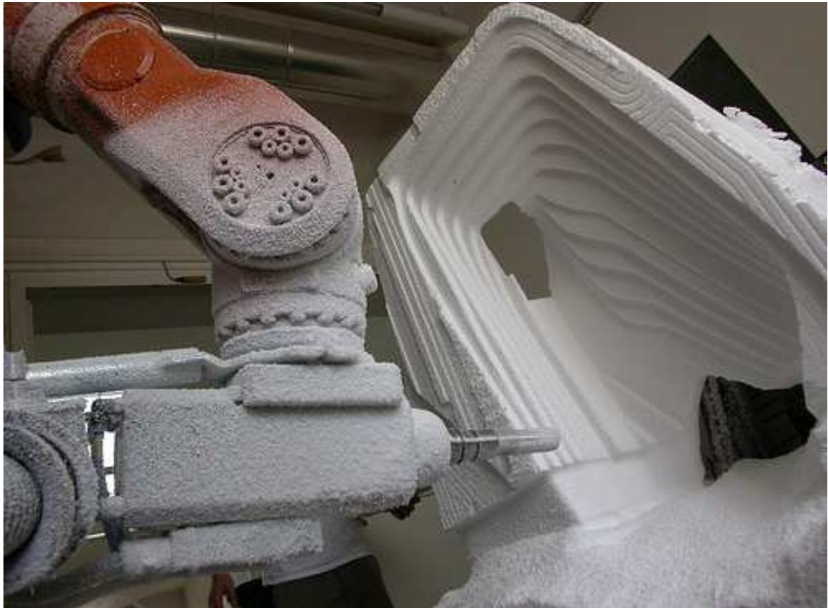
Fig.3 Kuka industrial robot cutting a path into foam. Lamp Prototype © SPAN 2008
